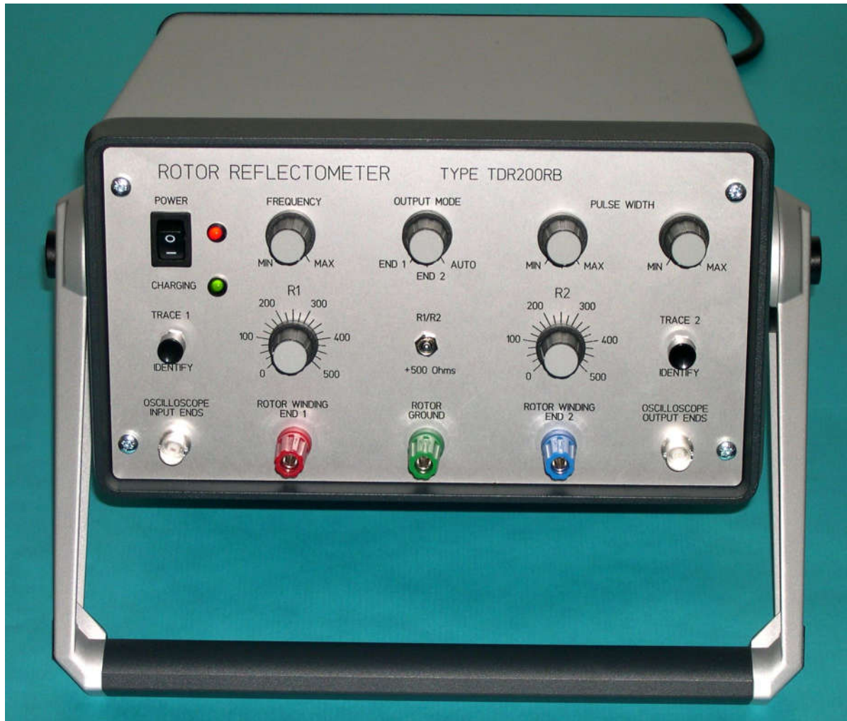
The TDR200 RSO Rotor Reflectometer
